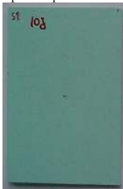
Figure 9: Plate subjected at impact with E = 10 J.
