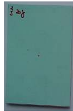
Figure 10: Plate subjected at impact with E = 20 J.
