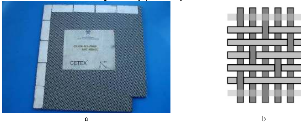
Figure 2: Studied samples: a) photo; b) scheme of 5HS carbon fiber woven
