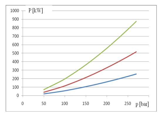
Fig.3. Theoretically available power for different pressure amplitudes with aperture diameter as parameter
