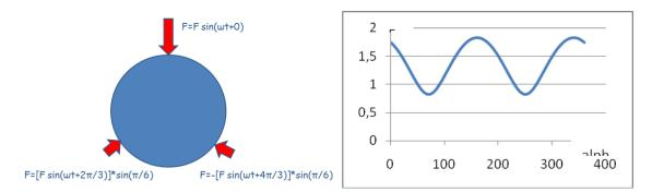
Fig.4. The mechanical model of the sonic asynchronous motor and the resultant rotor force The multi-domain model of the freewheel asynchronous model is given in figure 5.
