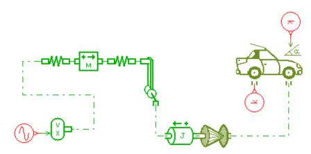
Fig.5. The multi-domain model of the freewheel asynchronous model
