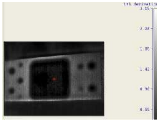
Figure 8: Thermogram obtained with first derivative representation.
