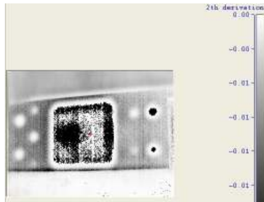
Figure 9: Thermogram obtained with second derivative representation.
