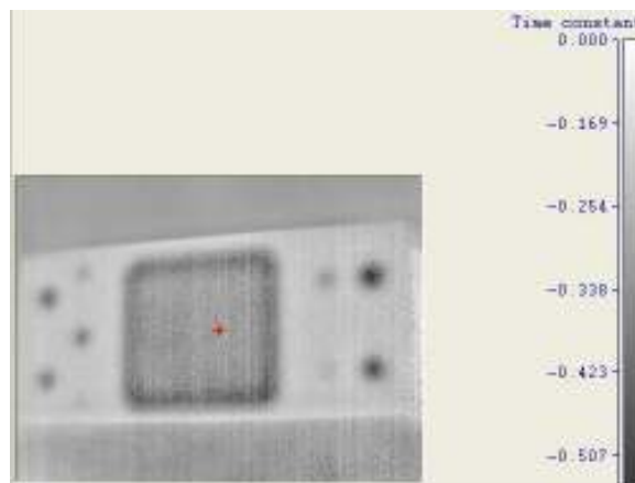
Figure 10: Thermogram obtained with time constant representation.
