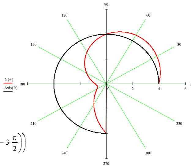
Fig. 7. Axial force diagram in polar coordinates
