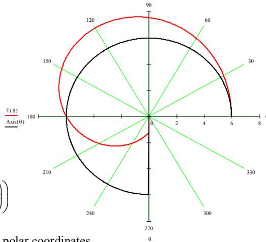
Fig. 6. Shear force diagram in polar coordinates
