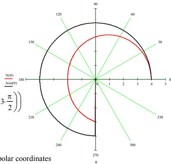
Fig. 3. Axial force diagram in polar coordinates
