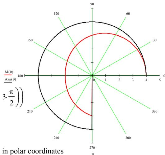
Fig. 4. Bending moment diagram in polar coordinates
