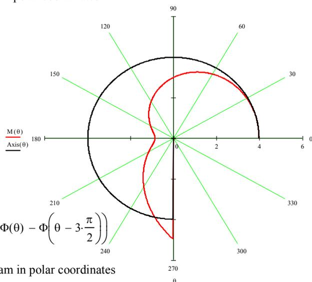
Fig. 8. Bending moment diagram in polar coordinates
