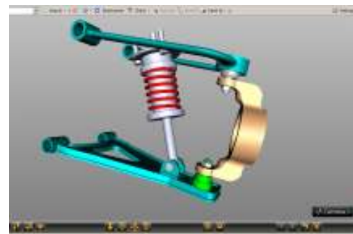
Figure 4: Auto front axle suspension mechanism connected to the virtual scene.
