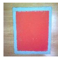
2 – finished thermo-system: wood fiber board, fiberglass mash, grout, primer, decorative finish with various granulations
