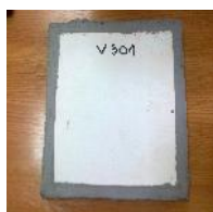
1 – finished thermo-system: wood fiber board, fiberglass mash, grout, primer, water based paint
