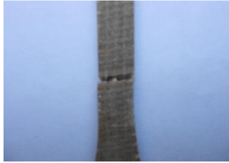
Figure 4. Resin specimens reinforced with hemp fiber, torn by traction
