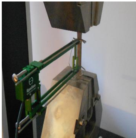
Figure 3. Tensile testing machine tried specimen mounted between the device terminals tensile test
