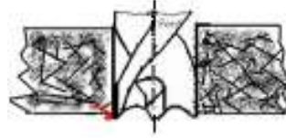
Figure 2: Push-out delaminating at exit
