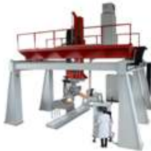
Figure 3: Fiber Placement Machine / Fiber Placement Detail
