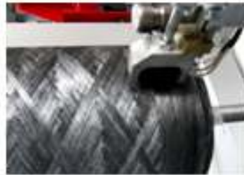
Figure 2: Filament Winding Machine / Detail of placement of roving over the mandrel
