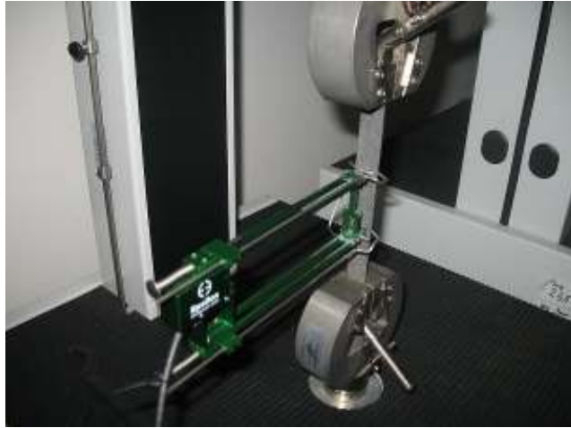
Figure 4: Tensile test detail on an epoxy impregnated 2/2 twill weave carbon fabric
