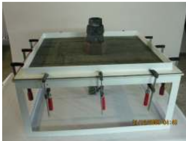
Figure 2: Flexural load-unload test detail. Sandwich panel clamped on contour
