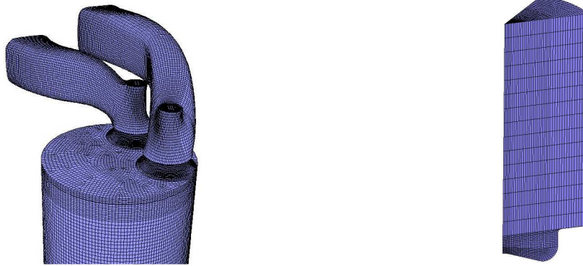
Hexahedral meshes for in-cylinder flow (left) and combustion (right) calculations
