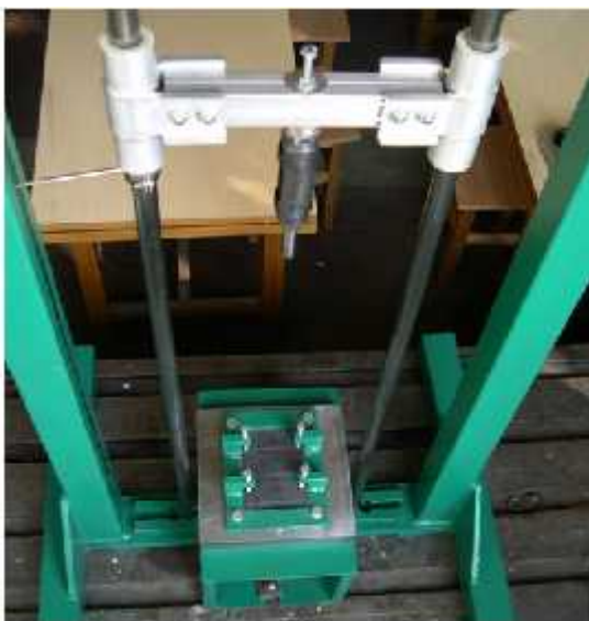
Figure 1 The device used to apply the load through free fall.
