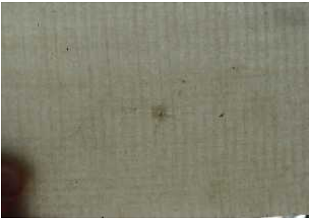
Figure 6. The damage resulted for a type A specimen - number 209 – subjected to an impact with an initial speed of the projectile of 2m/s.
