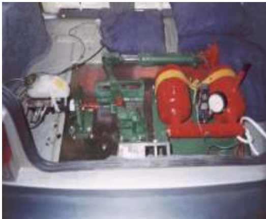
Fig 14. Adapted braking system of the motor vehicle
