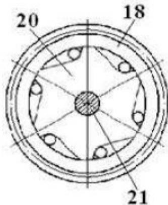
Fig.12. One way coupling with rotation way opposite to the one in fig.11, front view
