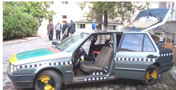
Fig. 10 Dismantling right front door to provide visual space for the dummy during rear collision
