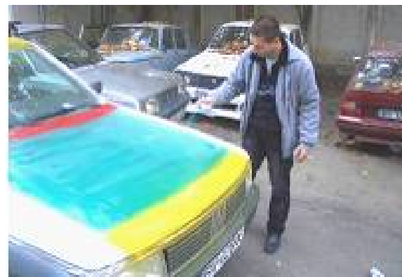
Fig.11 Painting on areas of the impact of the surfaces bodies vehicles
