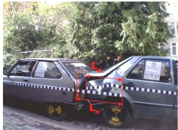
Fig. 18 Deformation measurement, the frame analysis
