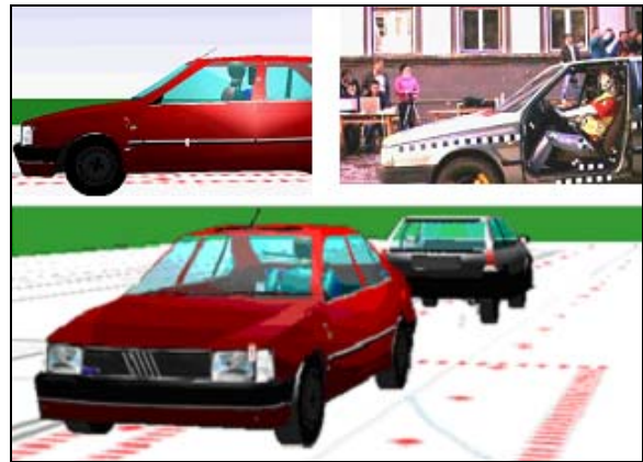
Fig. 2 Images of vehicle pushed, obtained from the PC-Crash and simulation video during the experiment
