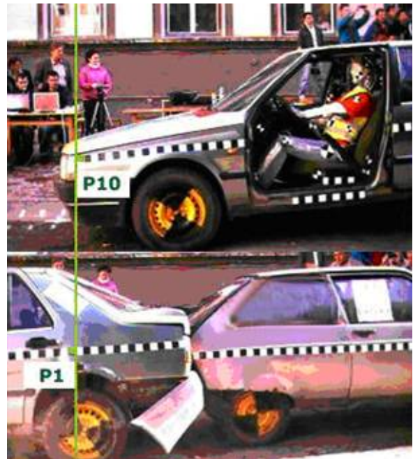
Fig. 17 Determining the covered distance by on the left side of the phused vehicle in video probe for v10= 26.4 km/h
