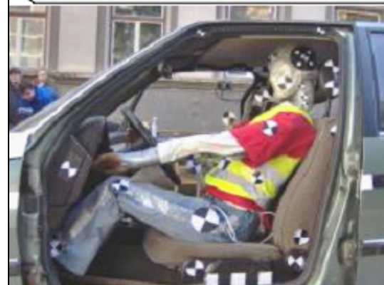
Fig. 14 Marking interior of the car
