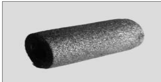
Fig. 2 The piston pin loaded by metal covering
