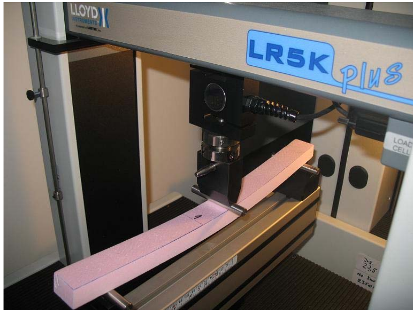
Figure 1: “LR5K plus” testing machine during the 3-point bending test of XPS foam
