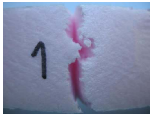
Figure 10: Irregular path of crack propagation in the outer surface of XPS foam specimen no. 1
