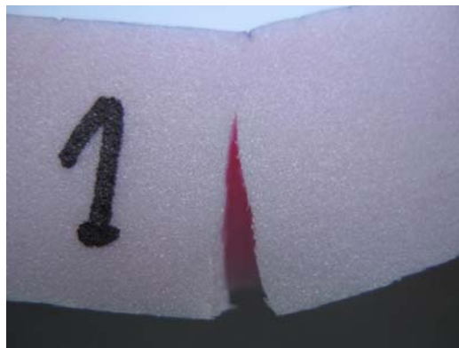
Figure 9: Crack beginning of XPS foam specimen no. 1
