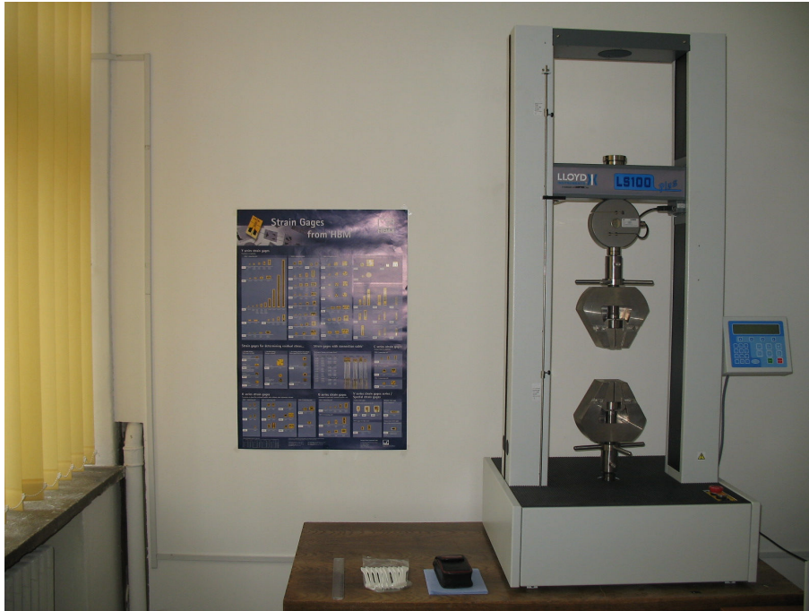
Figure 3: Lloyd's Instruments LS100 testing machine
