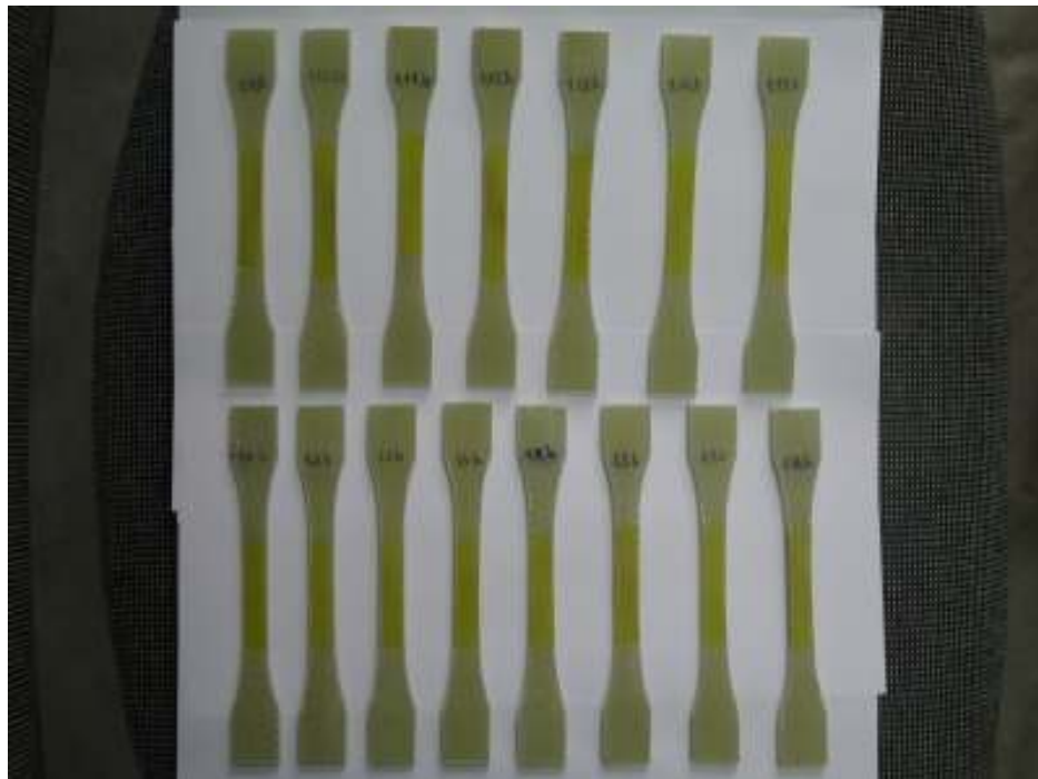
Figure 2: Specimens based on polyester resin reinforced with RT300 roving fabric
