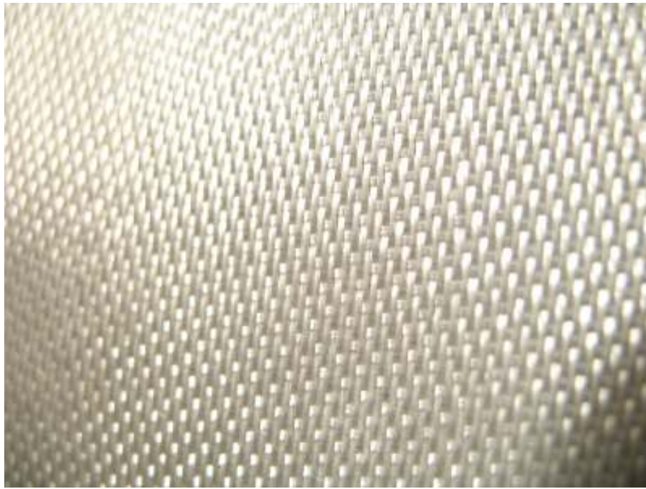
Figure 1: RT roving fabric reinforcement
