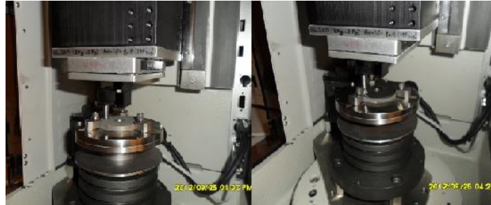
Figure 1: The way how the sampled is mounted on the CETR UMT-2 tribometre: a) the samples subjected to friction wear without lubrication; b) the samples subjected to friction wear lubrication.
