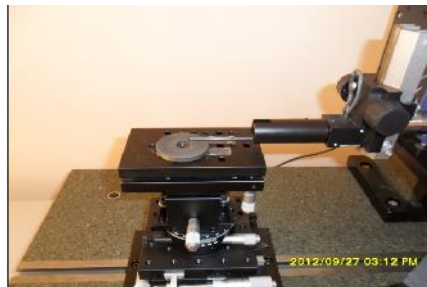
Figure 2: The mounting of the sample on the stand to determine the roughness of the profile
