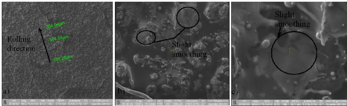
Figure 9: The appearance and dimension of the wear trace resulted after lubricated friction test: a) 80X, b) 1000X si c) 5000X
