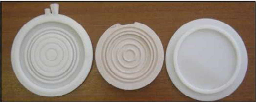
Figure 4: Upper VSD insert from silicone rubber manufactured in No 1 mould prototype
