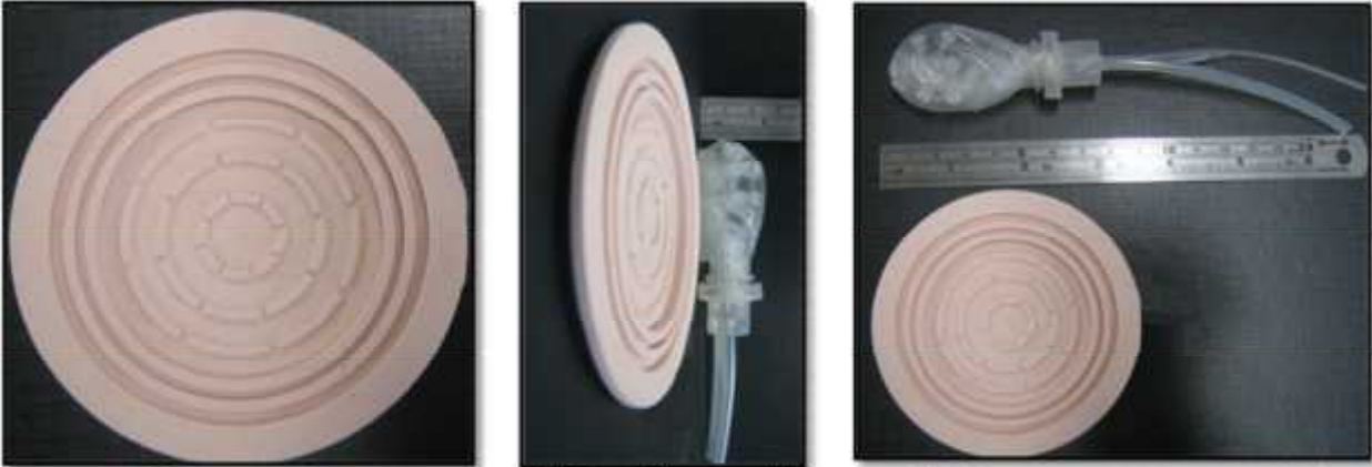
Figure 8: Upper VSD insert from mould prototype No 3
