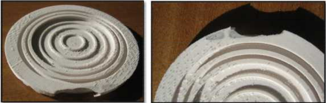
Figure 5: Flaws after the mould injection process
