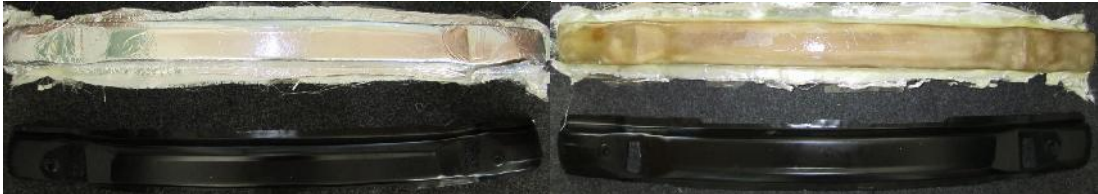
Figure 4: Bumper shock absorber made of composite materials removed from the mold [1]
