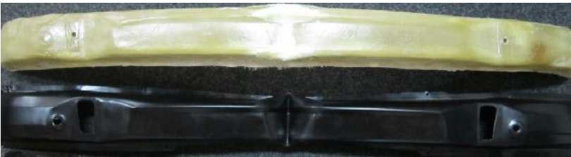
Figure 22: Black car bumper shock absorber made of steel and yellow car bumper shock absorber made of composite materials after impact testing[1]
