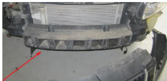
Figure 1: Car bumper shock absorber made from polystyrene [1]
