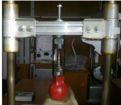
Figure 7: Device type slide with steel ball projectile
