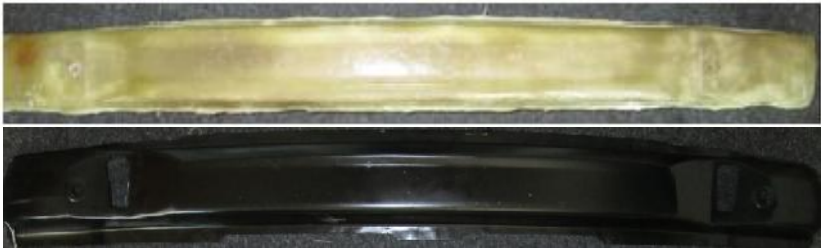
Figure 15: Black car bumper shock absorber made of steel and yellow car bumper shock absorber made of composite materials before impact testing [1]
