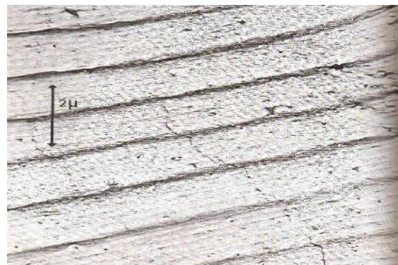
Figure 1b: The fatigue crack propagation front
