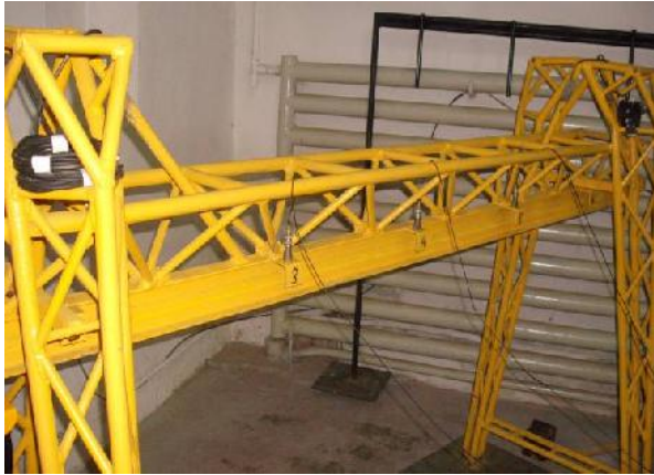
Figure 4: Scheme for the execution of the modal identification tests
