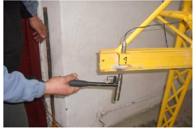
Figure 5: Test execution – detail of the excitation
