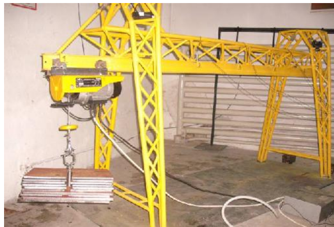
Figure 1: The connection scheme for the determination of the dynamic answer of the crane, due to the fracture of the drive cable
