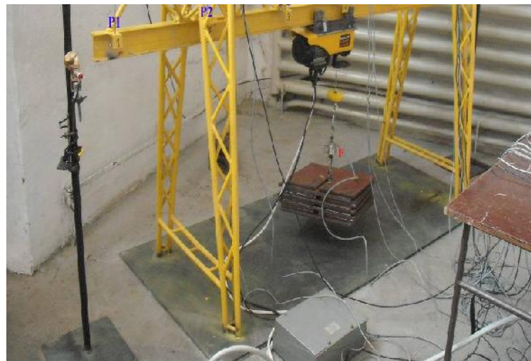
Figure 2. Assembling scheme for the deflections measurement
