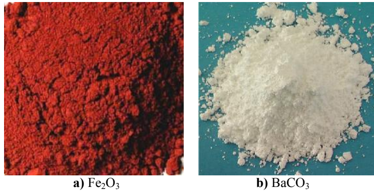
Figure 1: Fe 2 O 3 and BaCO 3 powders used for mechanical alloying process
