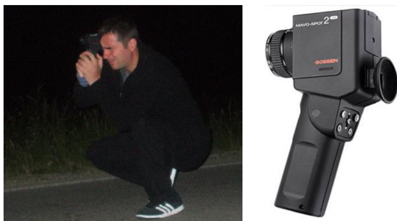
Figure 2: The use of lux meter GOSSSEN Mavo Spot 2
