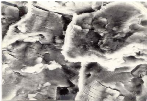
d. Fracture surface detail. The direction of crack growth at the level of material grains is evident (x3000)
