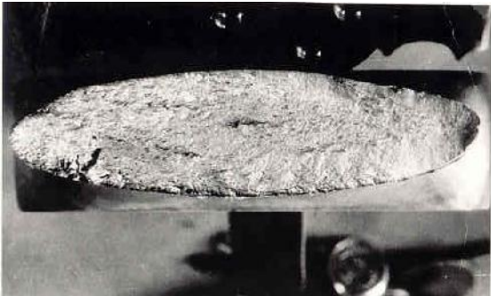
a. Cross section of the specimens subjected to fatigue
