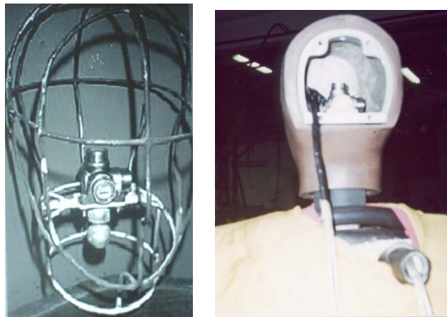
Figure 1. Accelerometer, mounted in head's CG (left). Dummy's head (right)
