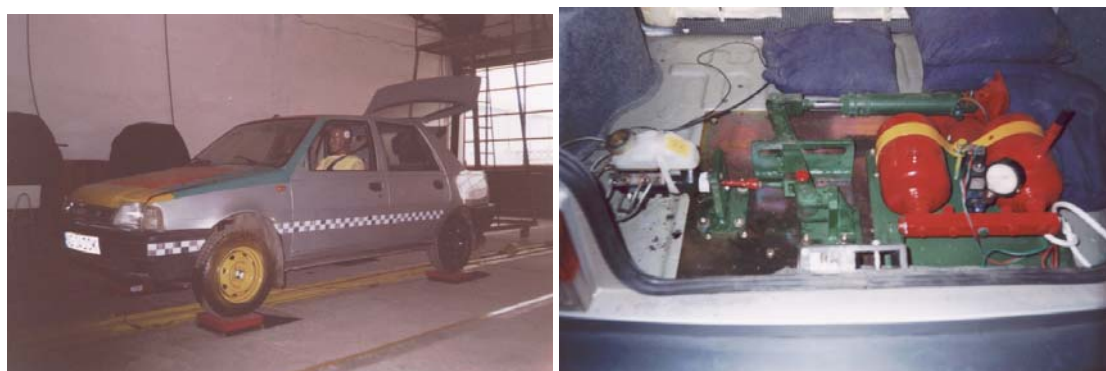
Figure 2. Weighing the test vehicle equipped with two humanoid dummies Hybrid II. (left) Braking system mounted on vehicle (right)
