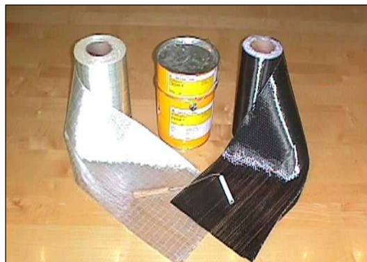
Fig.4 –CFRP sheets and adhesive.
