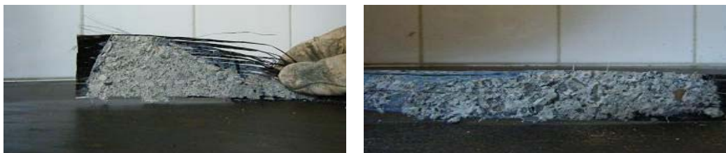
Fig.13 –Recommended detach between plates and concrete.
