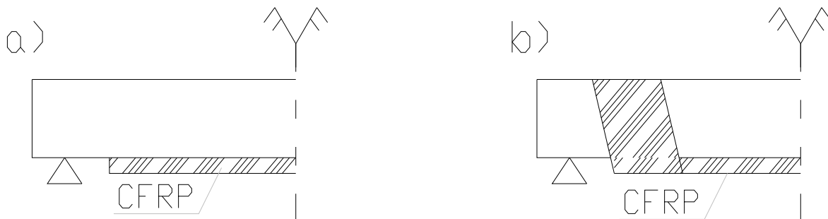
Fig.1- Detail of applying CFRP materials on beams.
