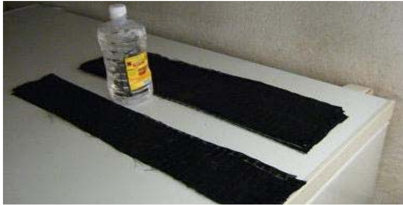
Fig.6 –Nitro solvent and CFRP sheets.
