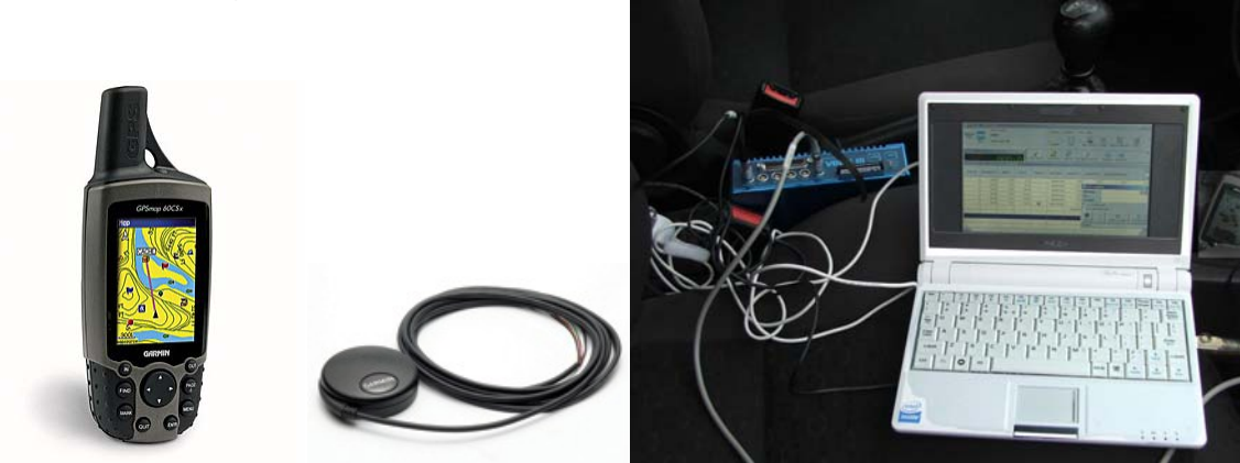
Figure 2: Three GPS devices used in measurements: left – Garmin GPSMap 60CSx; middle – GPS 18x-5Hz; right – Racelogic VBox (the blue case) and the first two devices
