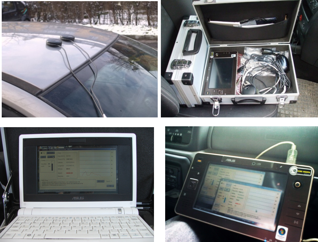
Fig. 4.5 – Complete acquisition system based on GPS 18x-5Hz
