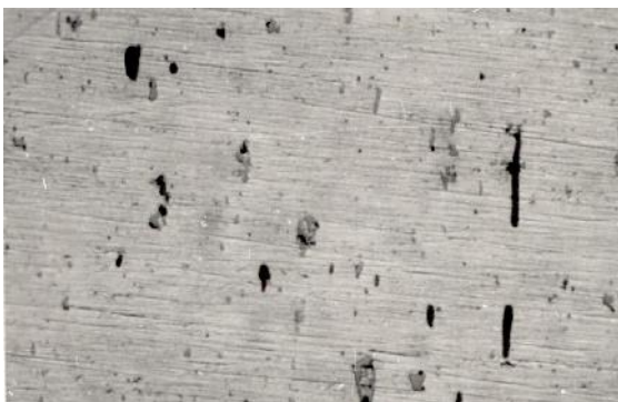
Figure 4: Microstructure of Al 6061 T651 (x300)
