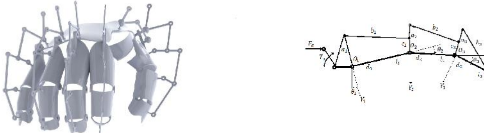
Figure 4: Virtual exoskeleton and four-bar linkage mechanism
