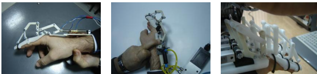
Figure 7: Exoskeleton structures and soft robotic glove
