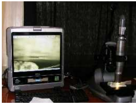
Figure 1: Keyence VHX-600 digital microscope (first two pictures) and mechanical testing system for dental samples
