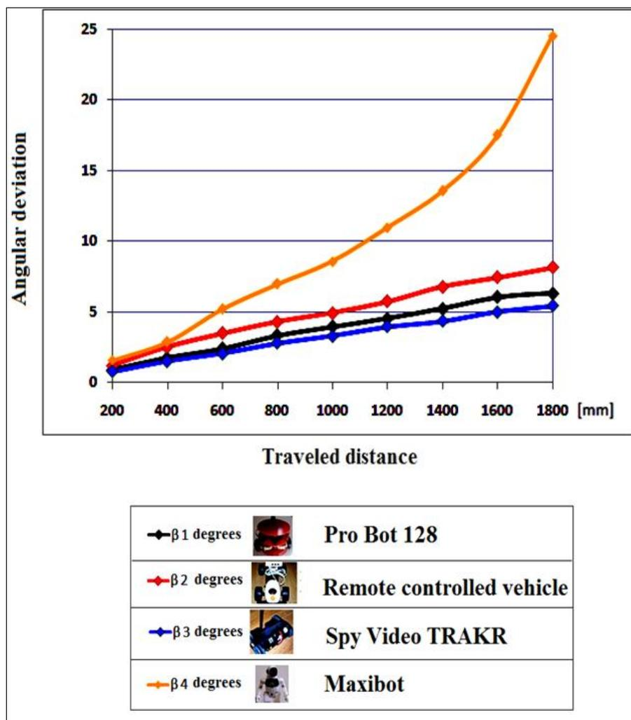
**Figure 7:** Angular deviation for the tested robots
