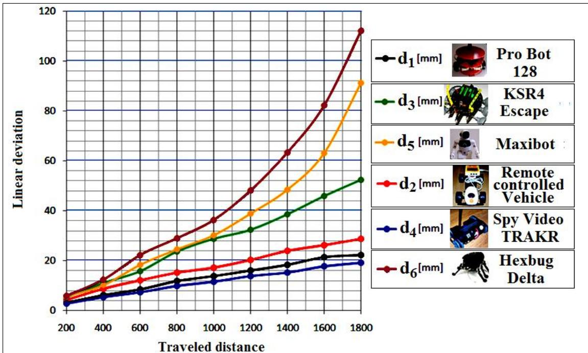
**Figure 3:** Linear deviation for the six mobile robots
