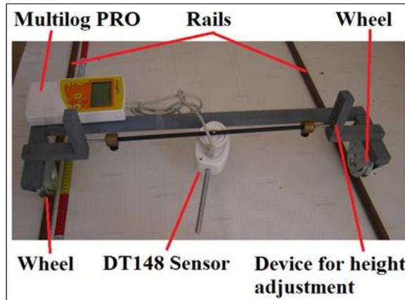
**Figure 5:** System for determining the angular deviation
