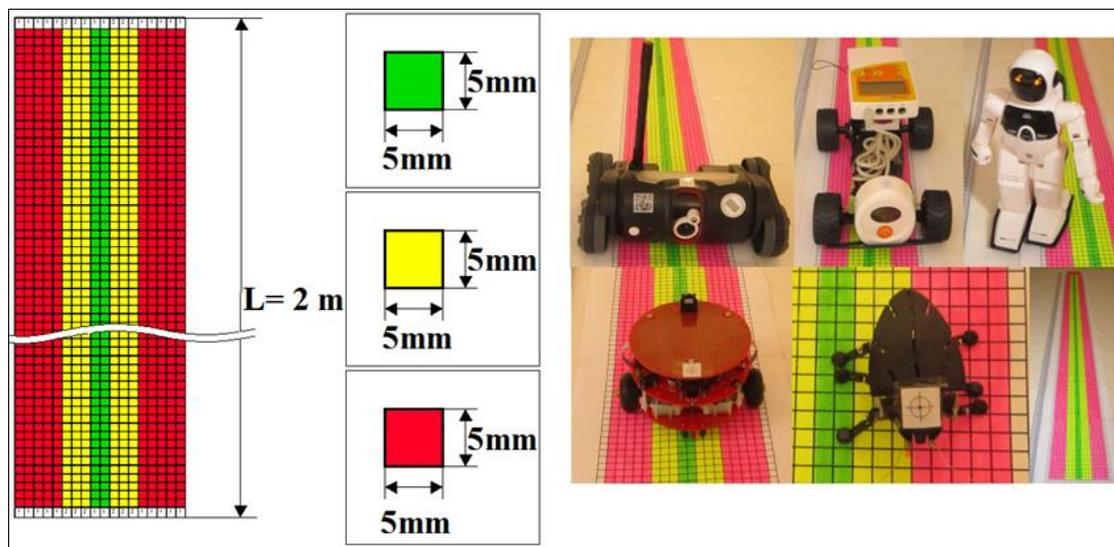
Figure 2: Trail chosen to determine the deviation from the trajectory
