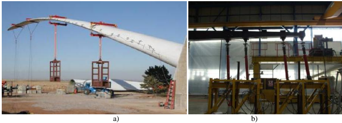
Figure 2: Static testing stand for blades of large dimensions: a) application of the force by means of weights; b) application of the force by hydraulic actuators [1]
