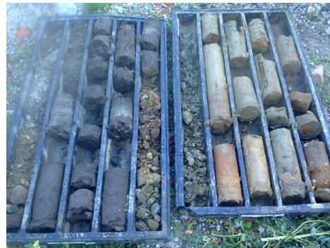
Fig. 2. The stratification identified in geotechnical borehole
