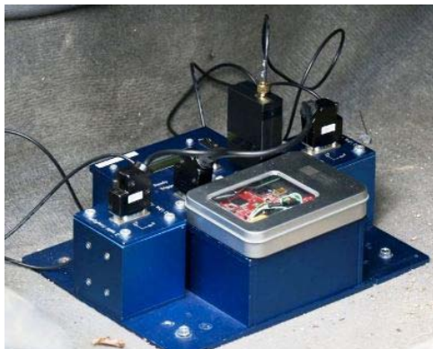
Fig. 4. PicDAQ on the vehicle floor, with Loka mounted on top of it
