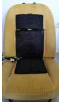
Fig. 3. Electric resistance heater
