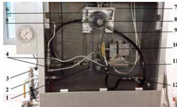
Fig. 3. Chain friction rig equipped with the guide friction device
