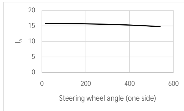
Fig. 9. Overall steering ratio (steering-wheel angle divided by road-wheel angle) as function of steering wheel angle
