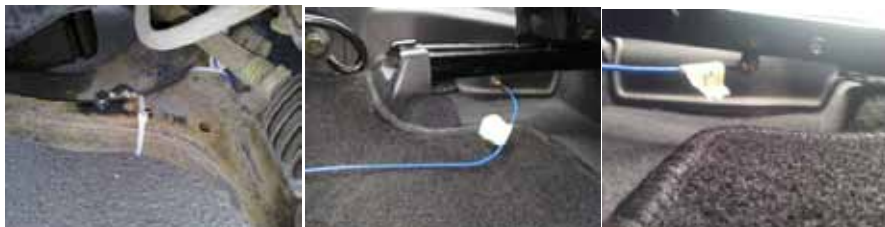
Fig. 5. Sensors location as following: lower control arm, left-seat and right-seat sliding rails
