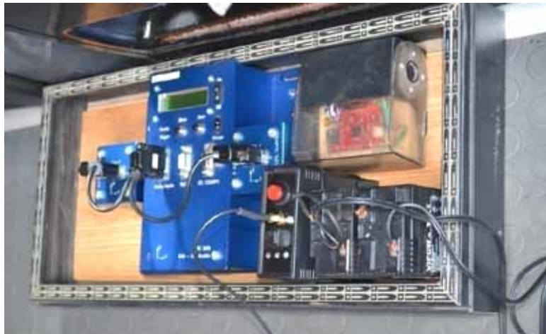
Fig. 5. PicDAQ, DL-10 and Loka units mounted on vehicle's floor
