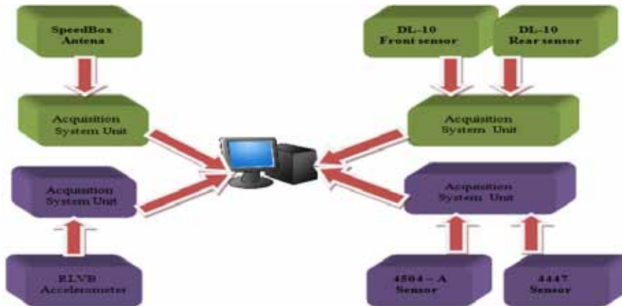
Fig. 11. The block diagram of data acquisition process
