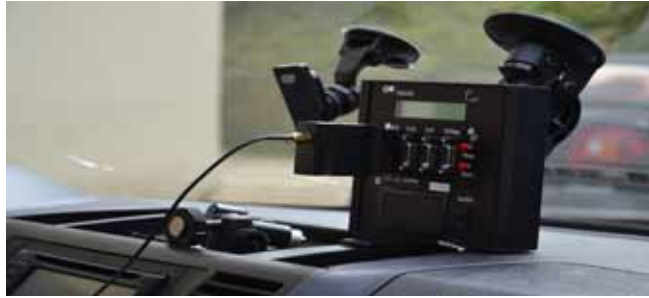
Fig. 4. PicDAQ - Inertial Measurement Unit
