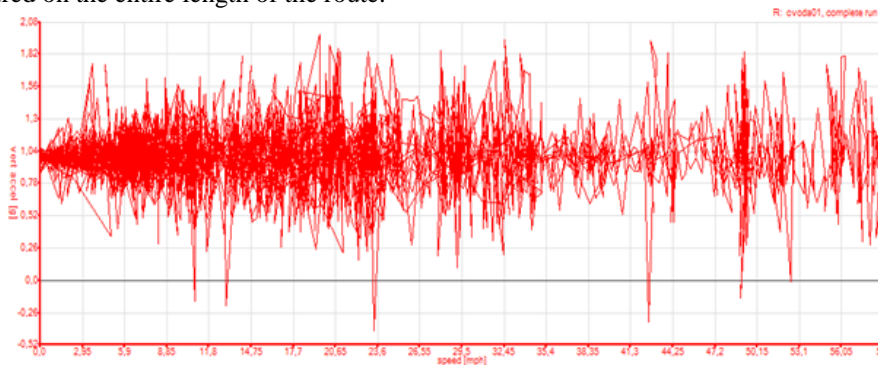
Fig. 9. The values of vertical accelerations, as a function of vehicle speed (Speedbox)
