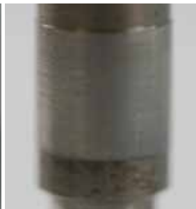
Fig. 6. Valve pin erosion
