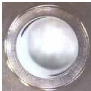
Fig. 4. Valve seat erosion
