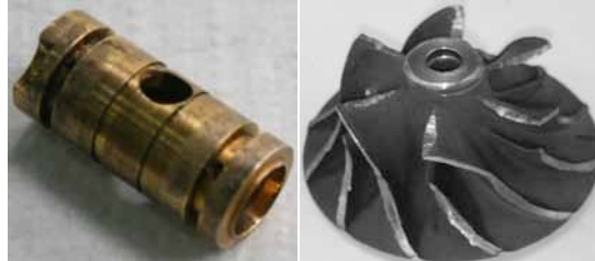
Fig. 2. Compressor wheel damage due to extreme journal-shaft clearance
