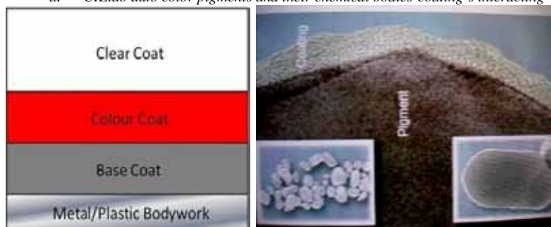
b. Minimum coverage succession of layers of bodies of cars (primer, color pigment paint, varnish)
