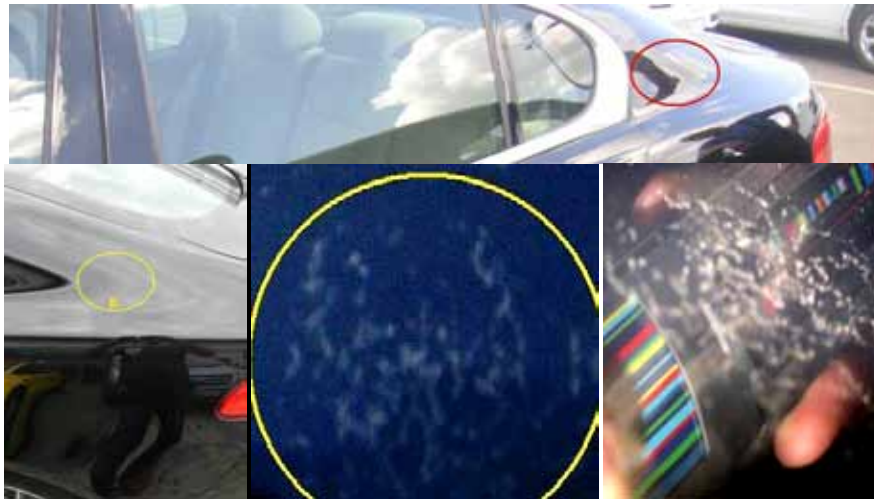
a. B Area b. paintwork coating damages lok like the "spider-net" type template
