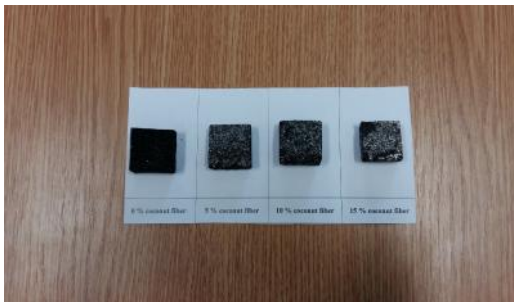
Figure 5: A complete set of samples for compression test
