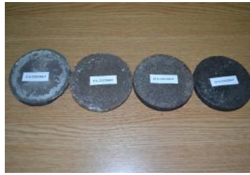
Figure 2: Finished composite samples with variable addition of coconut fiber
