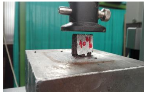
Figure 6: Sample with 10 % coconut fiber during compression tests
