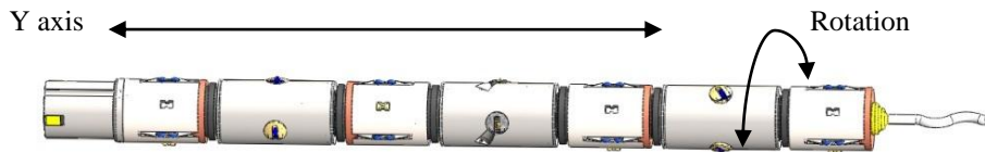
Figure 7: Schematic representation of the cutting and extraction device degrees of freedom
